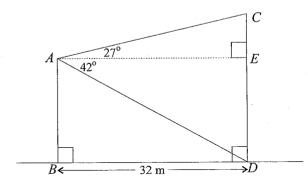
In the diagram above, two vertical buildings AB and CD are 32 metres apart. From A, the angle of elevation of C is  $27^{\circ}$  and the angle of depression to D is  $42^{\circ}$ .
